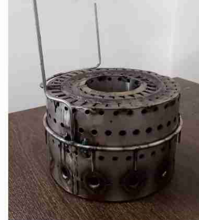
Combustion chamber and the fuel supply line
