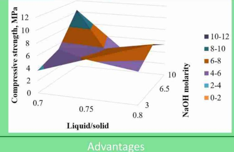
■ Raw materials: •Red mud; •Fly ash from the desulphurization process; Fly ash;
