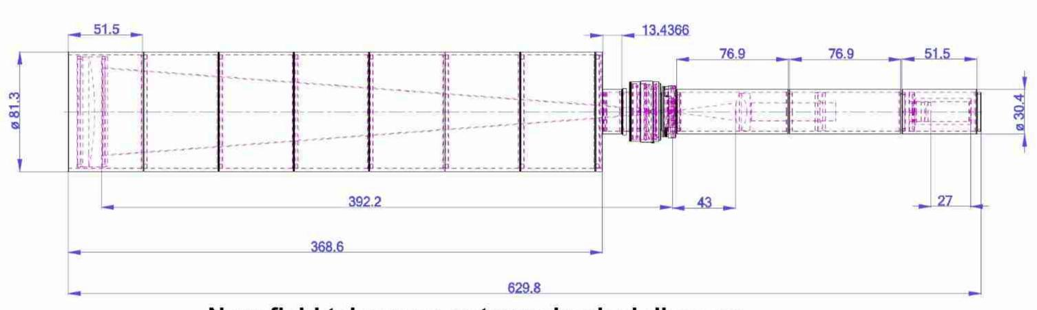
Near field telescope-optomechanical diagram
