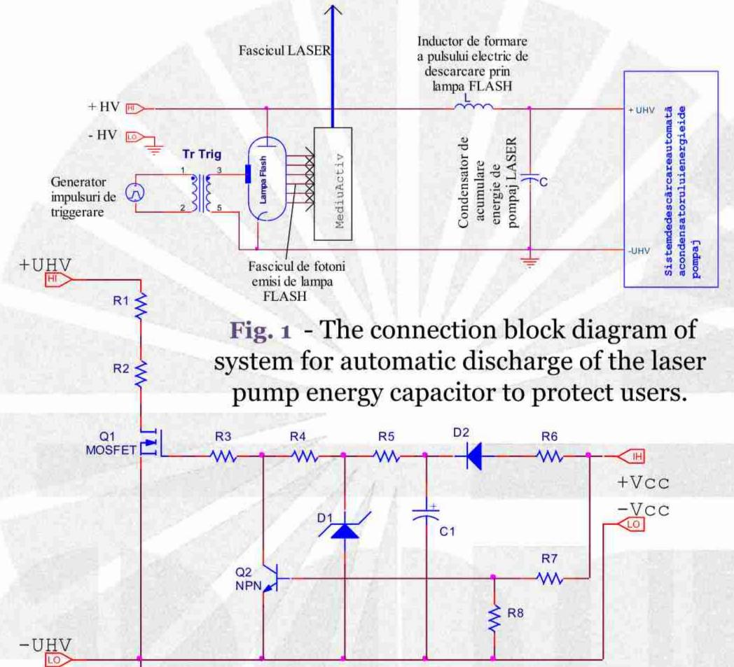
Fig. 2- Functional electrical diagram of the automatic discharge system of the laser pump energy capacitor to protect users.
