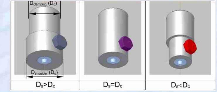
Variants of modular tool for friction stir welding and processing
