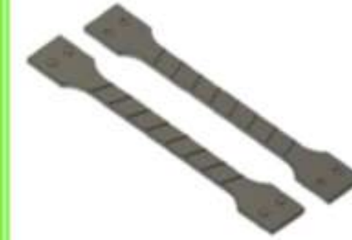
Test specimens resulting from PETG deposition
