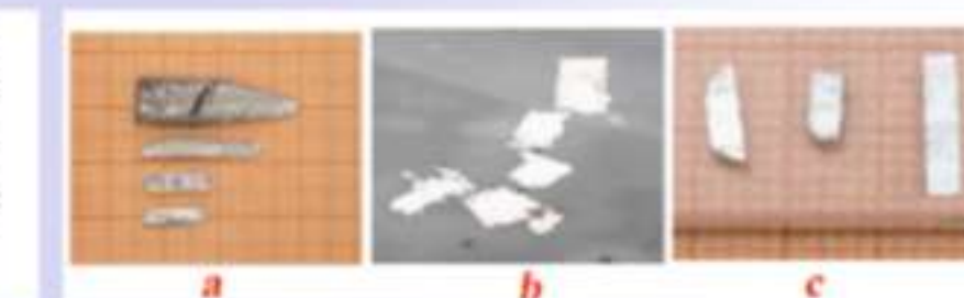
Fig. 3. Bulk Bi 2 Te 3 single crystal (a) Bi 2 Te 3 layer without substrate on the water surface (b) Bi 2 Te 3 layer without substrate on the graphite paper (c) Bi 2 Te 3 layer without substrate on the graphite paper.
